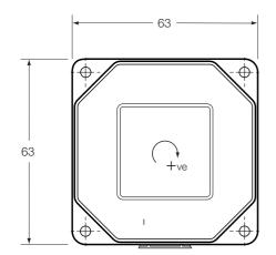
Connector: IL-S-8P-S2L2-EF (JAE) Mating Connector: IL-S-8S-S2C2-C (This connector with 500mm cable is included with each CRS09)
